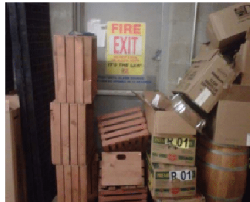
Figure 5-5: Lack of Safety Demonstrated by a Blocked Fire Exit
